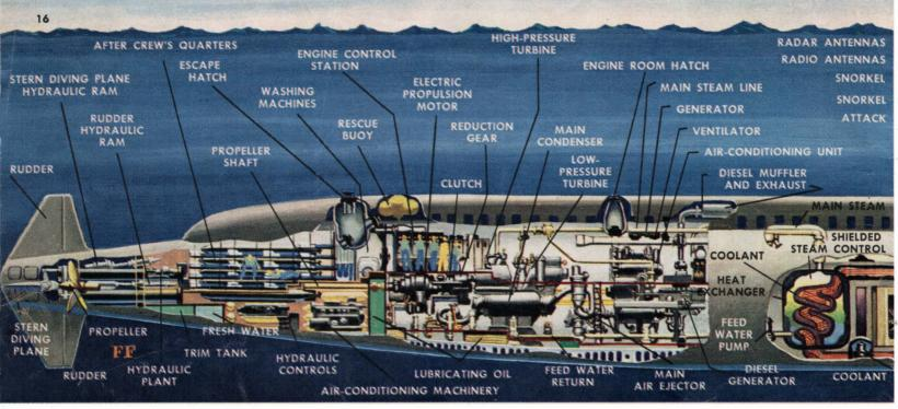
Cutaway shows location of the Nautilus' important units. Sub runs on atomic power, Diesel generators or batteries. The basic atomic power, heat
