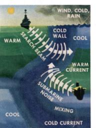
Composite diagram (l.) shows differing water densities that are caused in part by surface temperatures and warm and cold currents below the surface. Such variations in density give subs natural "hiding" places and chances for evasive tactics. Density variations deflect sound-search beams from surface vessels and any sound waves caused by submarine noises
