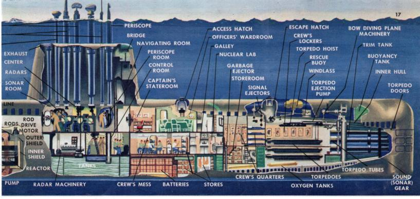
provided by reactor, is transferred to steam which turns turbines that drive propeller shaft
